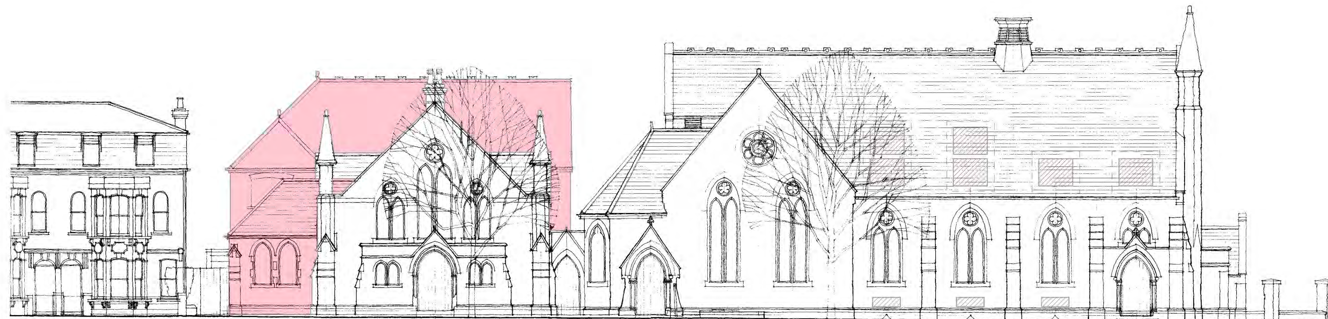
Demolitions South Elevation
